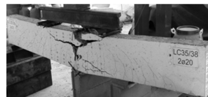
Fig. 3. Test beam after failure
